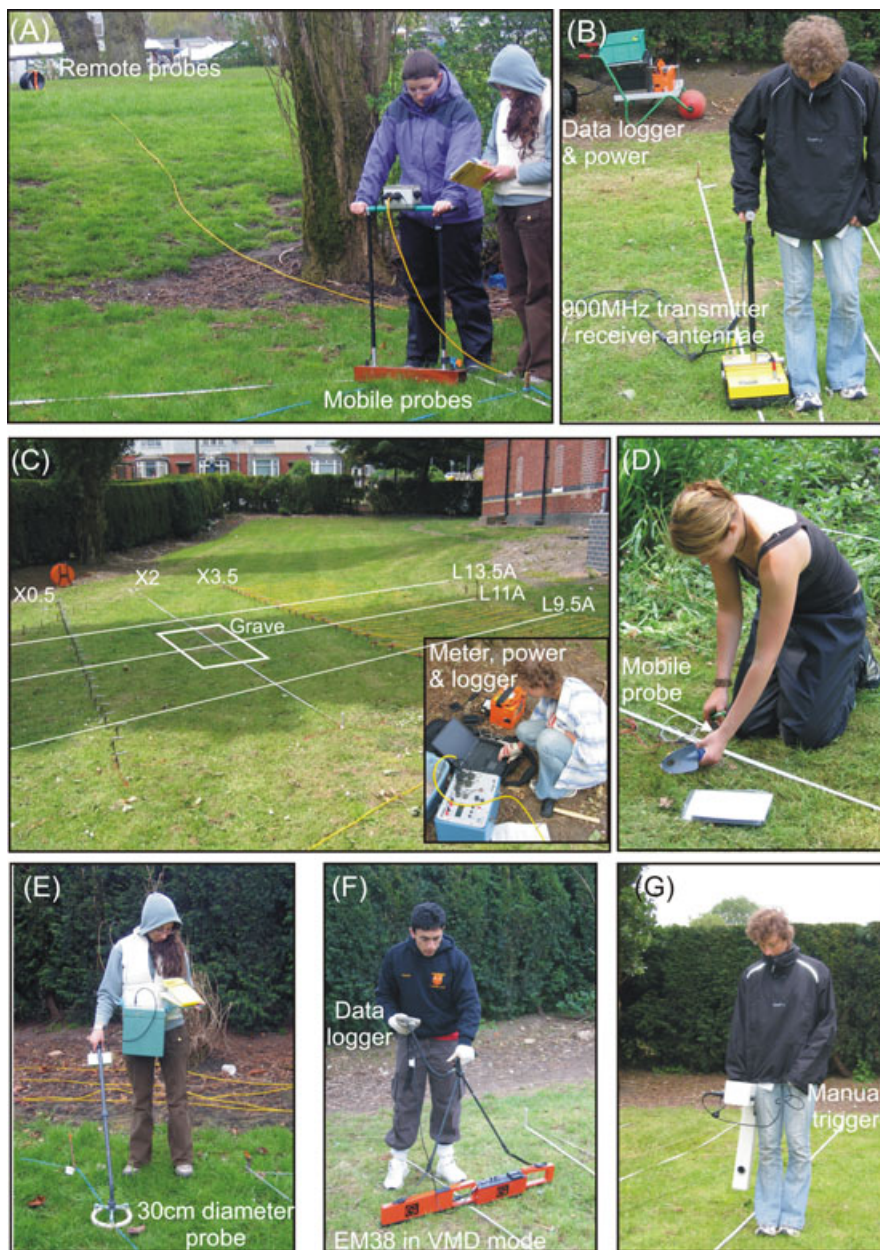
FIG. 3—Photographs of some near-surface geophysical equipment being trialled. (A) Bulk ground resistivity equipment; a Geoscan RM4™ lateral array. (B) High-frequency (900 MHz dominant frequency) GPR PulseEKKO™ 1000 equipment. (C) ERT electrode arrays ( \times 0.5 and \times 3.5 arrays laid out) using (inset) the CAMPUS TIGRE™ system. (D) SP survey using Pb-Cl probes and a standard voltmeter. (E) A Bartington MS.I™ magnetic susceptibility meter. (F) Bulk ground conductivity equipment: a Geonics EM38B™. (G) Magnetics equipment: a Geoscan FM18™ fluxgate gradiometer.
